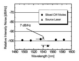
Fig. 7. Experimental results of relative intensity noise measurement. The results indicate that the longitudinal modes of the pump are replicated with 7 dB/Hz noise degradation. The results also show that each of the longitudinal modes can be carved to generate a CW signal. Uniformity of relative intensity noise shows that coherence is preserved equally across the SC.
