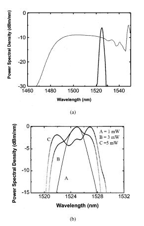
Fig. 3. (a) Transform limited pulse carving has been demonstrated vicinity of the EDFA band (1524 nm). (b) We check the propagation behavior of the carved pulses by propagating through 12 km DS fiber for three different input power levels. SPM dominated spectral modulation indicates that spectral carving of the SC near EDFA band generates soliton like pulses and coherence of the SC is maintained.
