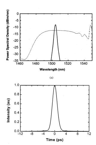
Fig. 4. (a) Transform limited pulse carving is demonstrated near 1500 nm. (b) The autocorrelation trace of the carved pulse at 1504 nm. We obtain 1.37 ps nearly transform limited Gaussian pulses with time-bandwidth product of  $\sim 0.45$ .
