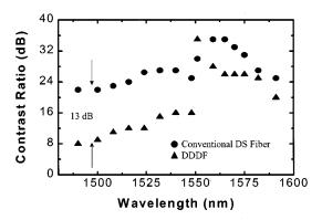
Fig. 9. Simulation results of the coherence degradation in short fiber SC generation and 1 km of dispersion decreasing and dispersion flattened fiber (DDDF). • indicates modulation depth (contrast ratio) of longitudinal modes calculated for SC generated in short DS fibers, and  $\triangle$  shows the contrast ratio calculated for the SC generated in long DDDF fibers. In average, short fiber SC generation has  $\sim 13$  dB higher contrast ratio than the one generated in 1 km fiber
