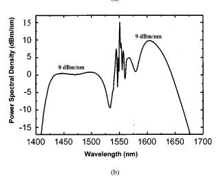
Fig. 2. (a) SC spectra generated in conventional DS fibers. We measure 140 nm bandwidth with  $\pm 0.5$  dB uniformity over 40 nm. Power spectral density is measured to be 7.9 dBm/nm over the flat region. (b) The spectral broadening improved to 250 nm with  $\pm 0.5$  dB uniformity over 83 nm by using high nonlinearity DS fibers.
